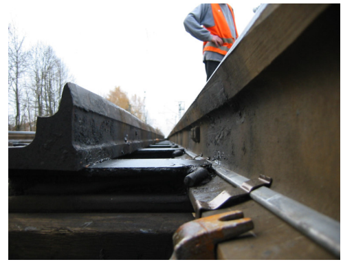
Position of heating element in free space between sliding seats and rail web
